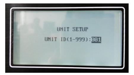
Press "UP" key or "DOWN" button to select the unit ID, then to power on the microphone unit, then press the speech button, about 5 seconds after the completion of the unit to return to the standby state, the host LCD display "set up to complete" and enter the next unit set up interface. At this point, you can continue to set the ID for more units, or press the "EXIT" button to exit the setting state, the system will return to standby mode.
