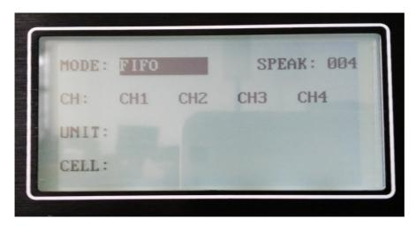
Press the "UP" or "DOWN" button to select the required mode, and then press the "ENTER" button to determine and save, the system will return to standby mode. If you choose the "TIME LIMITED" mode, continue to set the hours, minutes, and seconds. As shown below:
