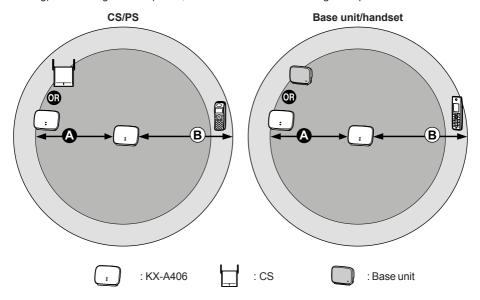
Repeater coverage area for synchronization between CS/base unit/destination repeater and repeater.
