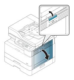
3. Remove the jammed paper from the exit unit or fuser unit.
