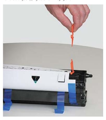
4. Remove remaining shipping tape and pull protective sheet from imaging unit.
