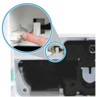
**CAUTION:** Make sure the connector is fully seated in the socket.
