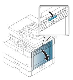
2. Remove the jammed paper from the transfer roller assembly.
