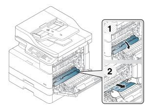
3. Open the fuser jam cover and remove the jammed paper.
