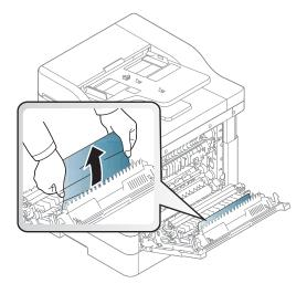
3. Release the transfer roller assembly and remove the jammed paper.
