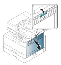
2. Open the jam guide and remove the jammed paper.
