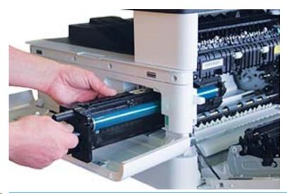
NOTE: If imaging unit binds or does not slide easily into cabinet, verify the right door is fully open, realign imaging unit, and install.
