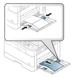
In the software application, set the margins to at least 6.4 mm (0.25 inches) away from the edges of the material.
