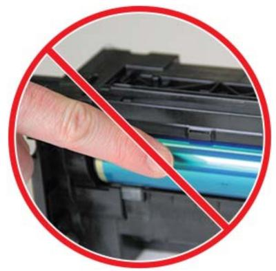
NOTE: Do not expose the imaging unit to light for more than a few minutes.
