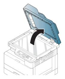
4. Grasp the misfeed original, and remove the paper from the feed area by carefully pulling it.
